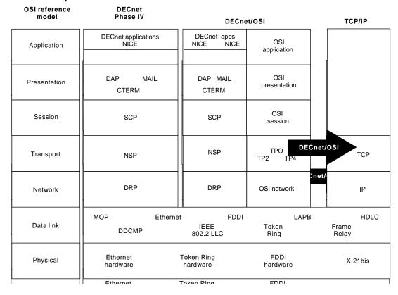
Figure 38-6 DECnet Phase IV and DECnet/OSI Support the Same Data Link and Physical Layer Specifications
